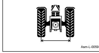
Add rear wheel weight, rear ballast box or implement. Make sure there is 25% of total weight on rear axle.
